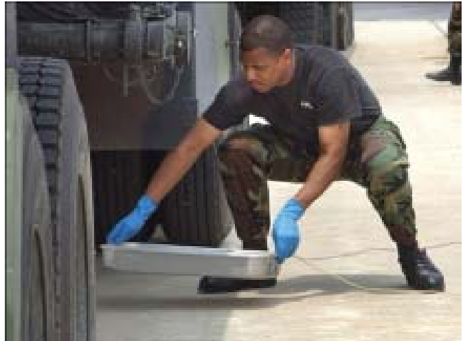
Senior Airman Karl White places a drip pan under the fuel connection during the exercise. Photo by Master Sgt. Sydney Fuchs, 108ARW/Visual Information Center.
